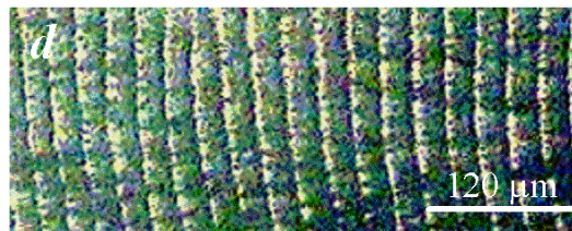
Figure 1. Polarizing optical microscopic texture formed by banana-shaped liquid crystals.
