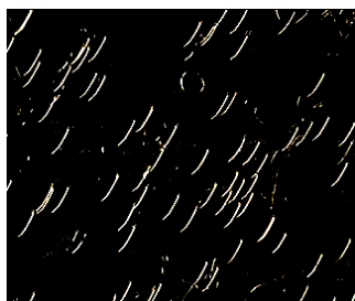
Figure 1. Micro photo of NC layer with thickness 1.8 \mu\text{m} made with crossed polarizers at room temperature. The size is 500 \mu\text{m} \times 400 \mu\text{m} .
