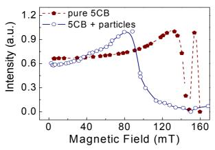
The Fréedericksz transition threshold for colloid appeared to be lower than that for pure LC. This fact shows that addition of magnetic nano-particles liquid crystals, which forms in colloid, influences the LC properties. The determined magneto-optical characteristics of the colloid proved be significantly increased to corresponding comparing to properties of the nematic matrixes.
