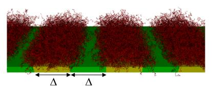
Three distinct morphologies of the nanopatterned brush have been identified and their range of stability has been determined in terms of a single universal parameter  $\xi = \Delta / N \sigma_s^{1/3}$  that combines the grafting density, the polymer length and the stripe width. Under good solvent
